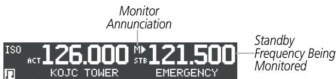
Standby COM Frequency Monitor Annunciation
